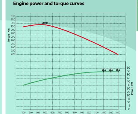
Engine speed, RPM
